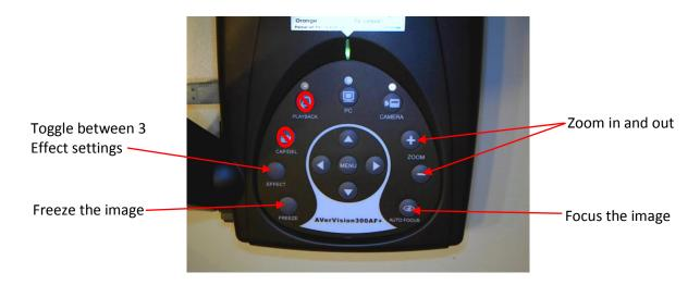
6. Remote Control (the labeled buttons are the only ones functional when set up through a USB connection)
